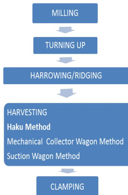
Figure 2.29 The process of peat harvesting and the three most common peat production processes
