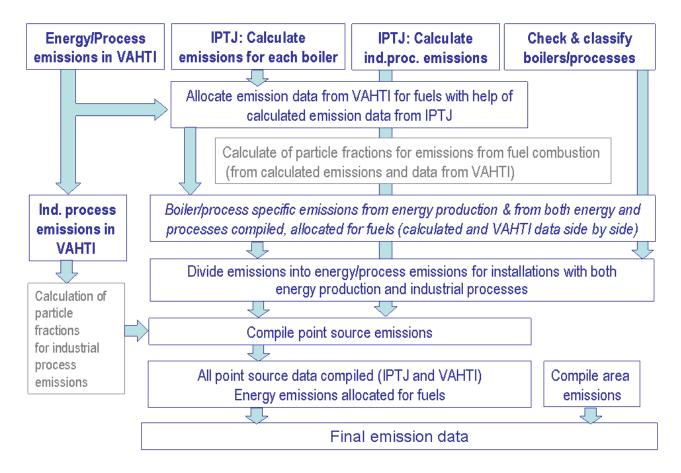
Figure 1.10. Processing of emission data reported by the plants for use in the air pollutant emission inventory, Part 2. (Note; the name of VAHTI has been changed to YLVA in 2018)
