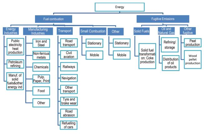
Figure 2.1. Emission sources included under the Energy Sector in the Finnish air pollutant inventory.
