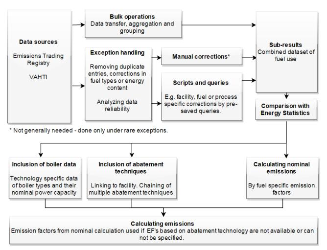
Figure 2.14. The process of calculating emissions from combustion plants
