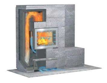
Figure 2.23. Air flow in a masonry oven (Alakangas et al 2008)
