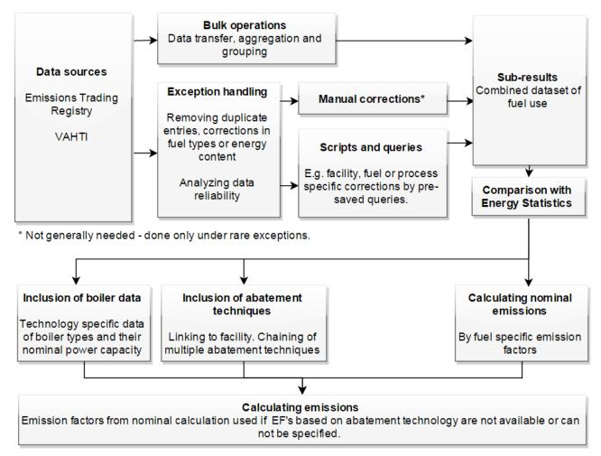
Figure 2.14. The process of calculating emissions from combustion plants
