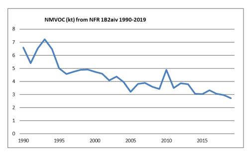
Figure 2.33 NMVOC emissions from refining/storage
