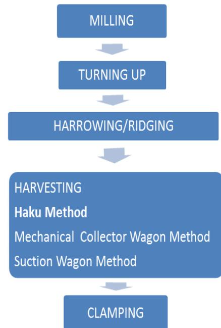
Figure 2.32 The process of peat harvesting and the three most common peat production processes
