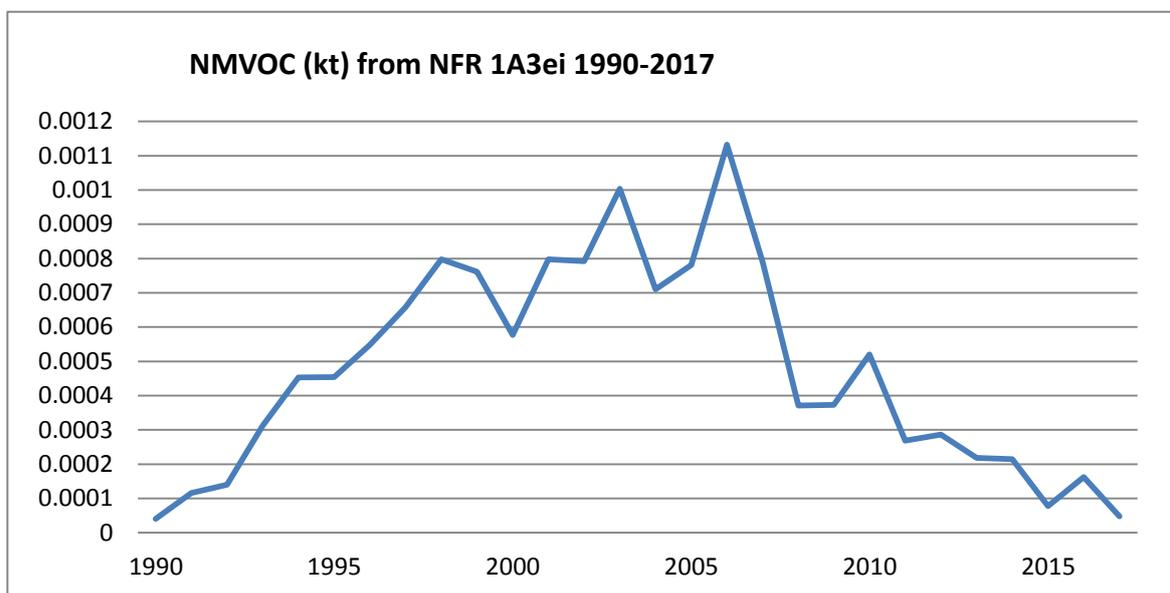
Figure 3.16 NMVOC emissions from pipeline compressors 1980-2017
